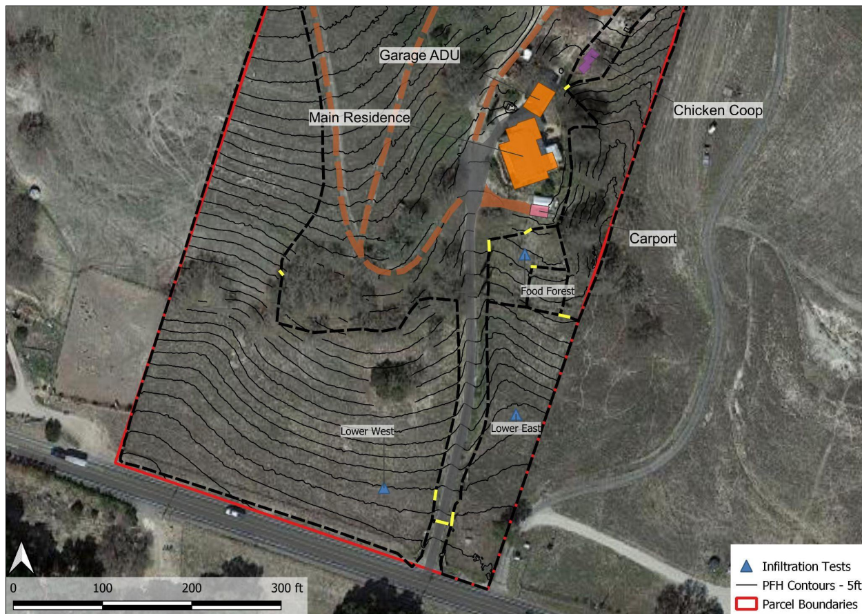
Figure 1.5.3 PFH infiltration test locations.
