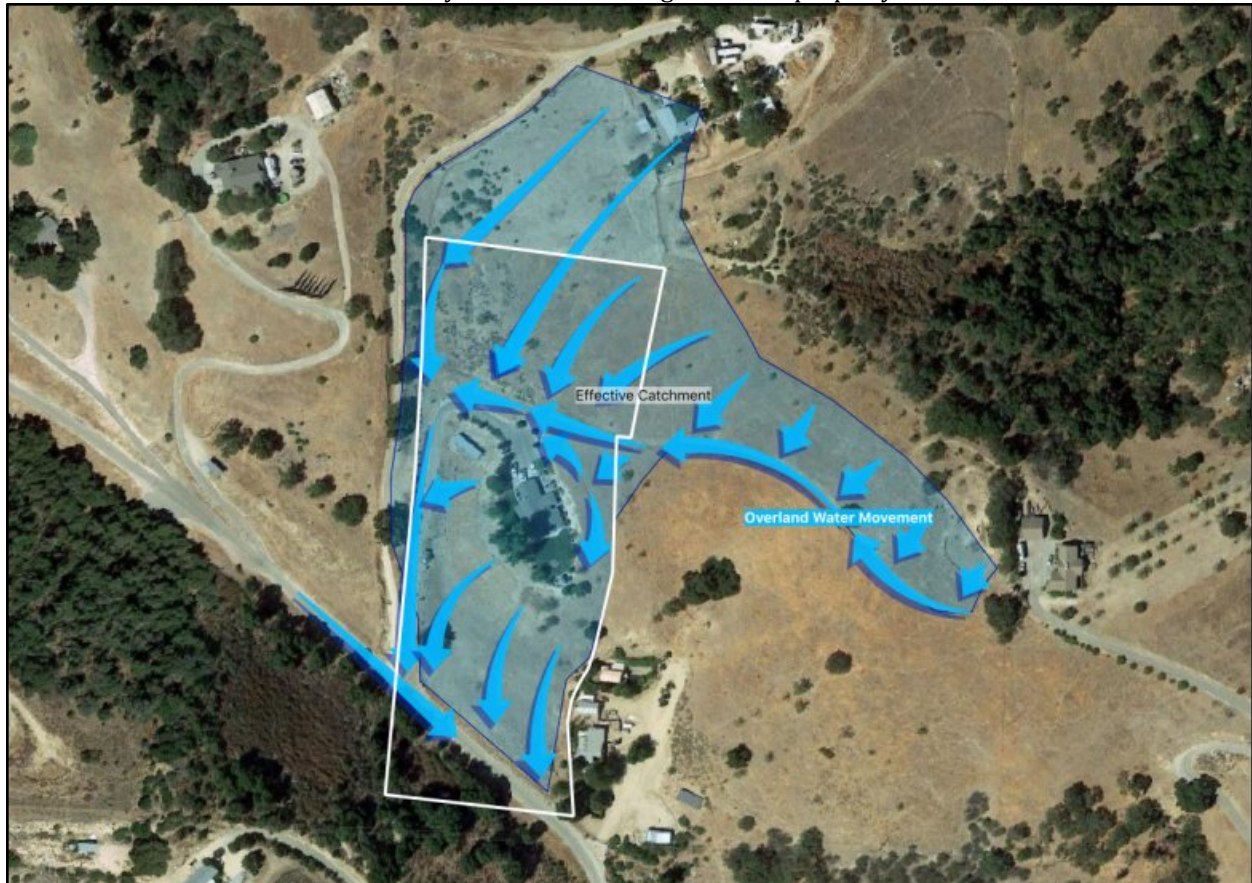
Figure 2.0.2 Primary watershed feeding into WFH property
